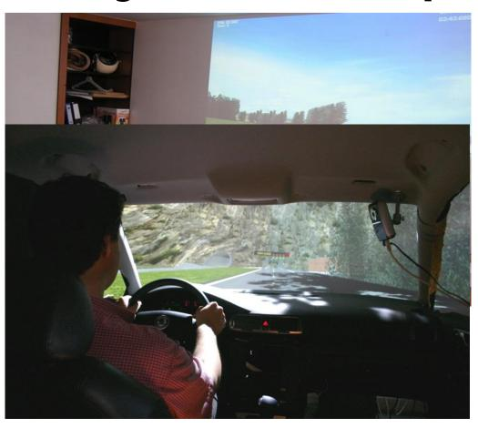
The first simulator based on Skoda cockpit
